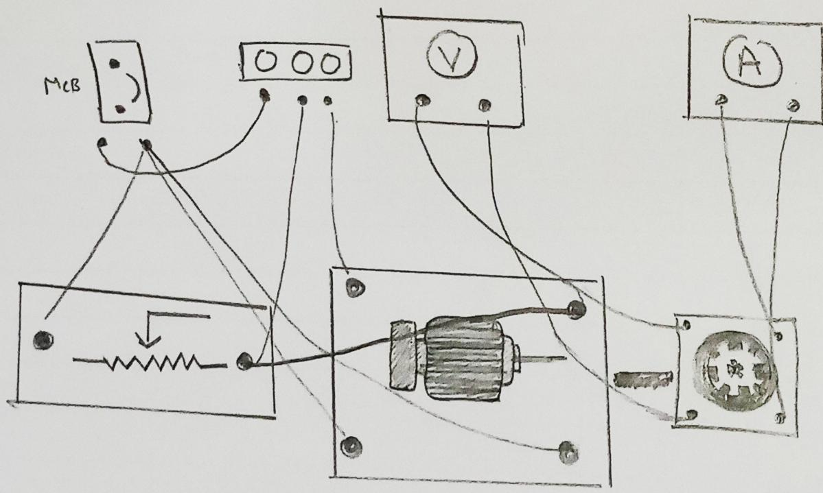
Aim: To study the magnetization characteristic of DC shunt generator. Draw the graph between the armature voltage & field current.
